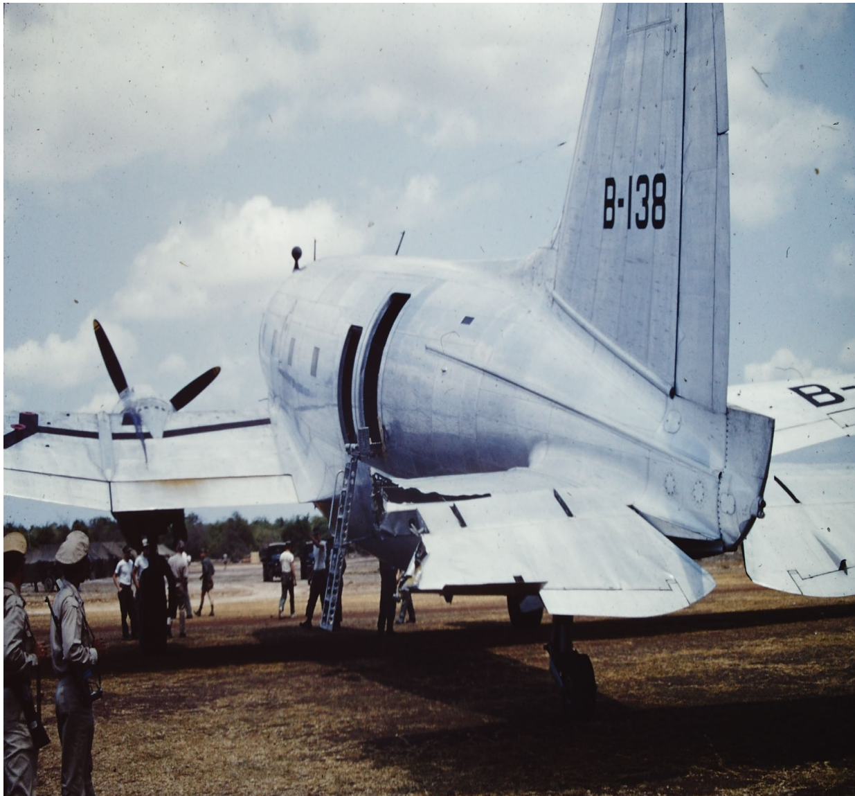
Air drops could be dangerous at times. The left elevator of Curtiss C-46F B-138 seen here was damaged during a cargo drop. The crew managed to return the ship to Wattay Airport for repairs. Clarke Collection.
