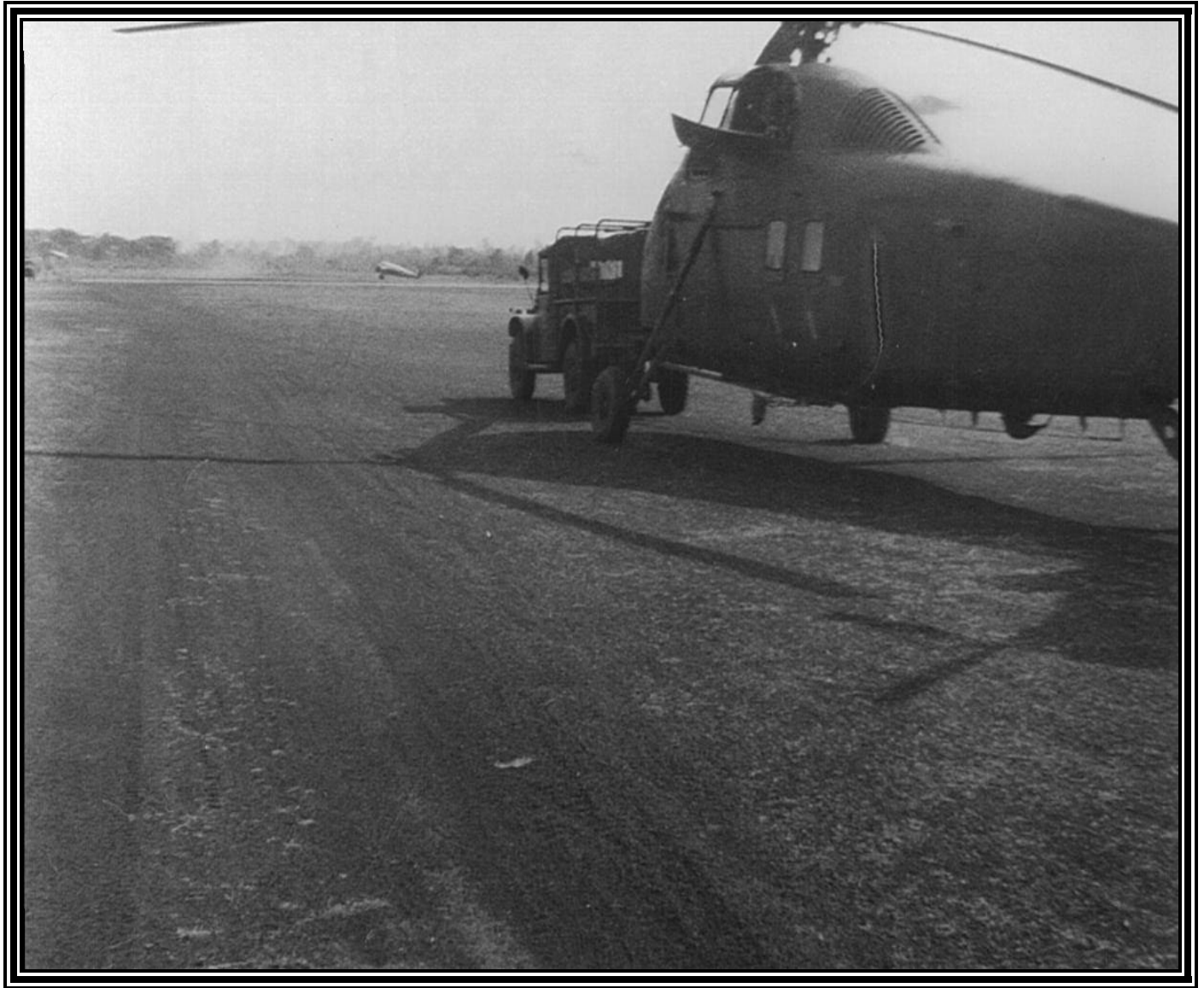
An Air America HUS-1 helicopter being towed by a weapons carrier along the laterite ramp to a parking spot in preparation for a test flight. Transmission deck platform is down for inspection. Dust from a taxiing aircraft is visible toward the end of the ramp.
