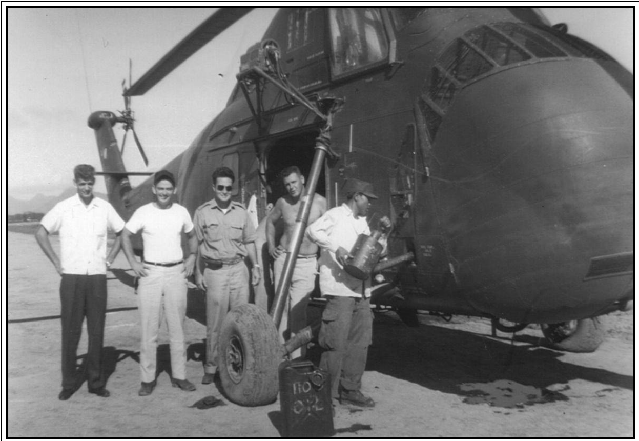
Oil change with Lao helper adding 1100 weight oil to the reservoir of a UH-34D R-1820 engine at Luang Prabang, Laos. Left to right: Unknown Flight Mechanic, Pilots Fred Sass, Dominic "Gooch" Gucchione, and shirtless Flight Mechanic Bert Palmer.
