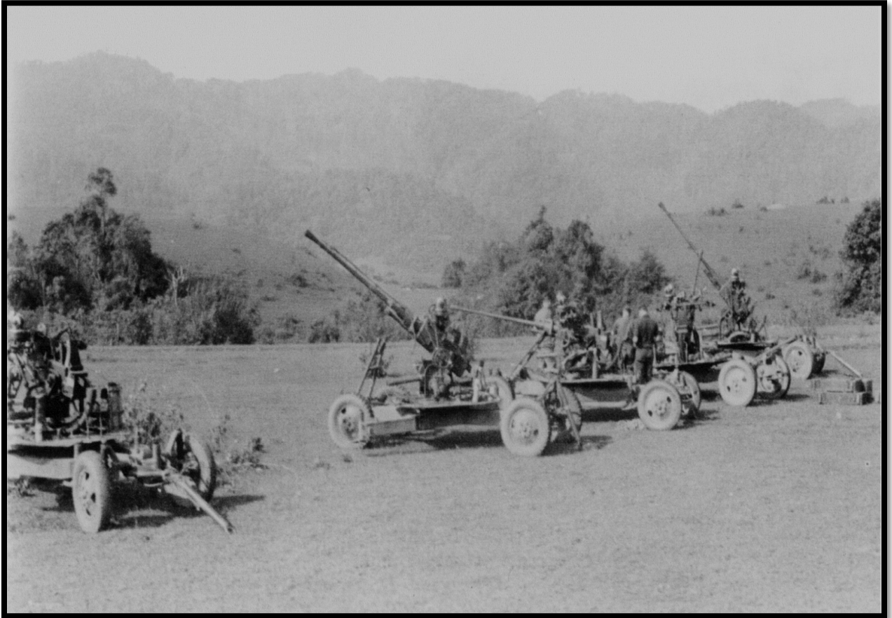
A portion of captured mobile Soviet 37mm anti-aircraft guns lined up at Xieng Khouang Ville, Laos.
