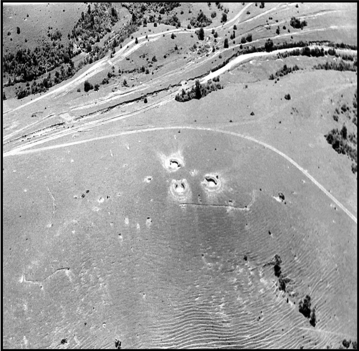
Three horseshoe shaped 37mm gun pits perched on a hill in the Xieng Khouang Vile Valley. Radar controlled AAA could be directed from a van placed in the center of the earthen revetments.
