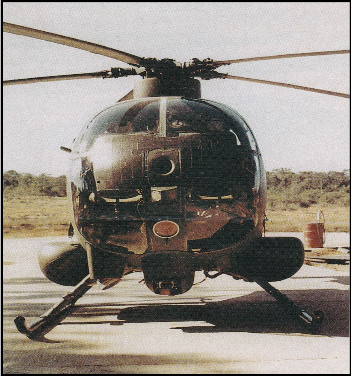
Front view of the mission-oriented Hughes-500P displaying side pods containing sensitive electronic navigation equipment. The pod underneath the belly was reserved for the forward-looking-infra-red (FLIR) system.
