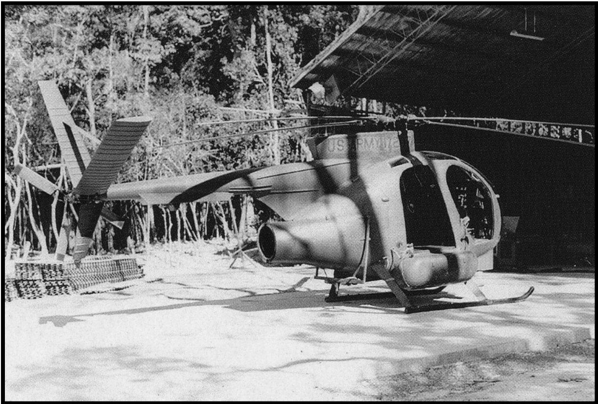
Right side view of a U.S Army version of the relatively silent H-500P showing additional drive components, reinforced skids, and external pods for housing navigational and associated equipment.
