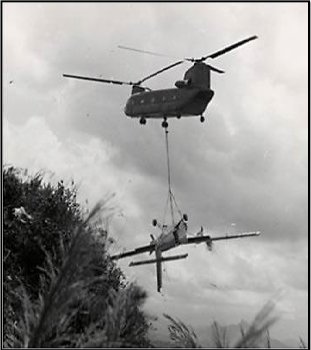
Captain Billy Pearson and his crew lifting DHC-6 N389EX with Chinook 016 from a hillside below the LS-260 airstrip.
