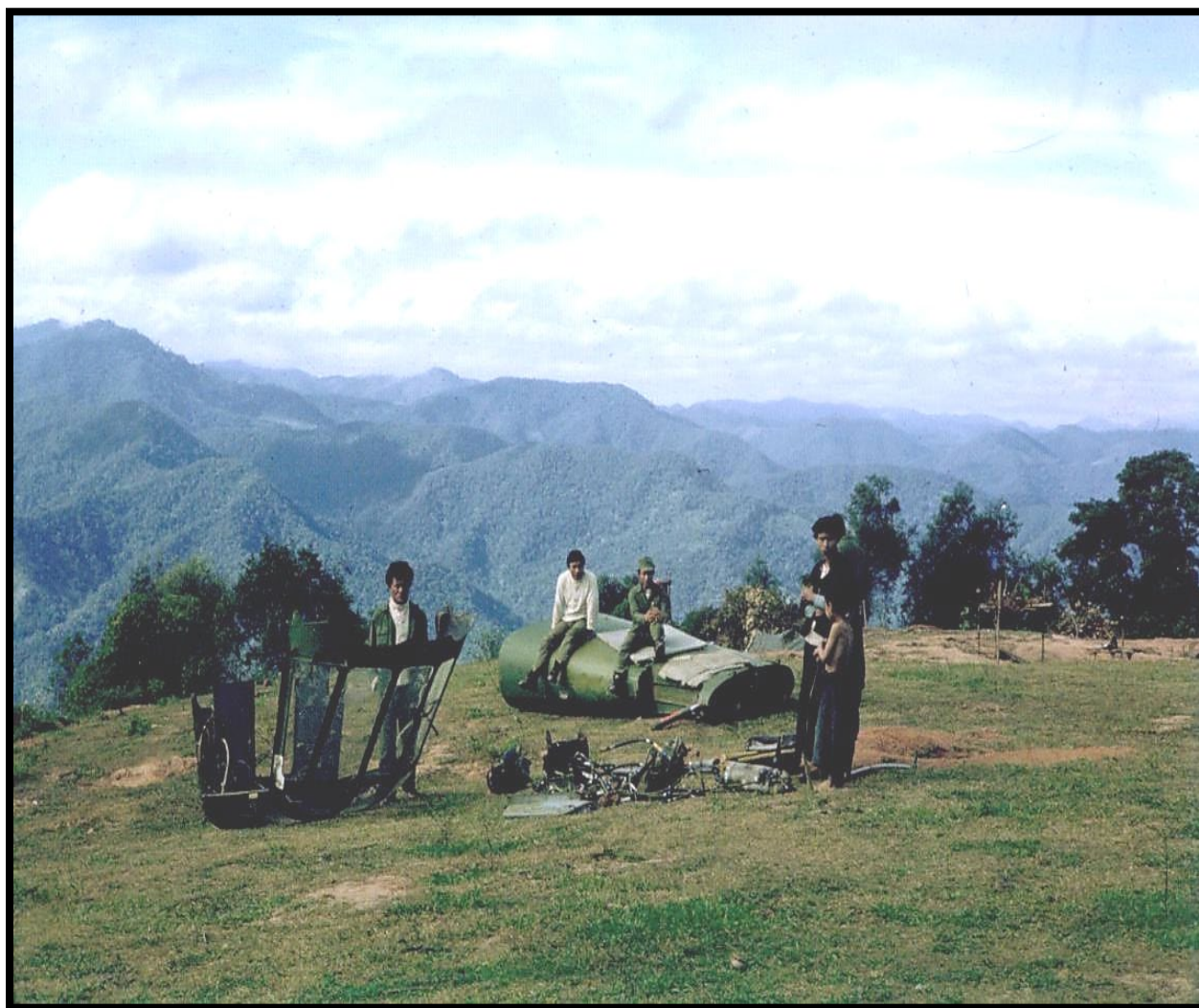
A collection of parts from the Hotel-30 crash sitting at Mak Phout (LS-137) for delivery to Udorn. They include: a tail cone, upper portion of the forward cockpit section, and various smaller parts. Nichols Collection.
