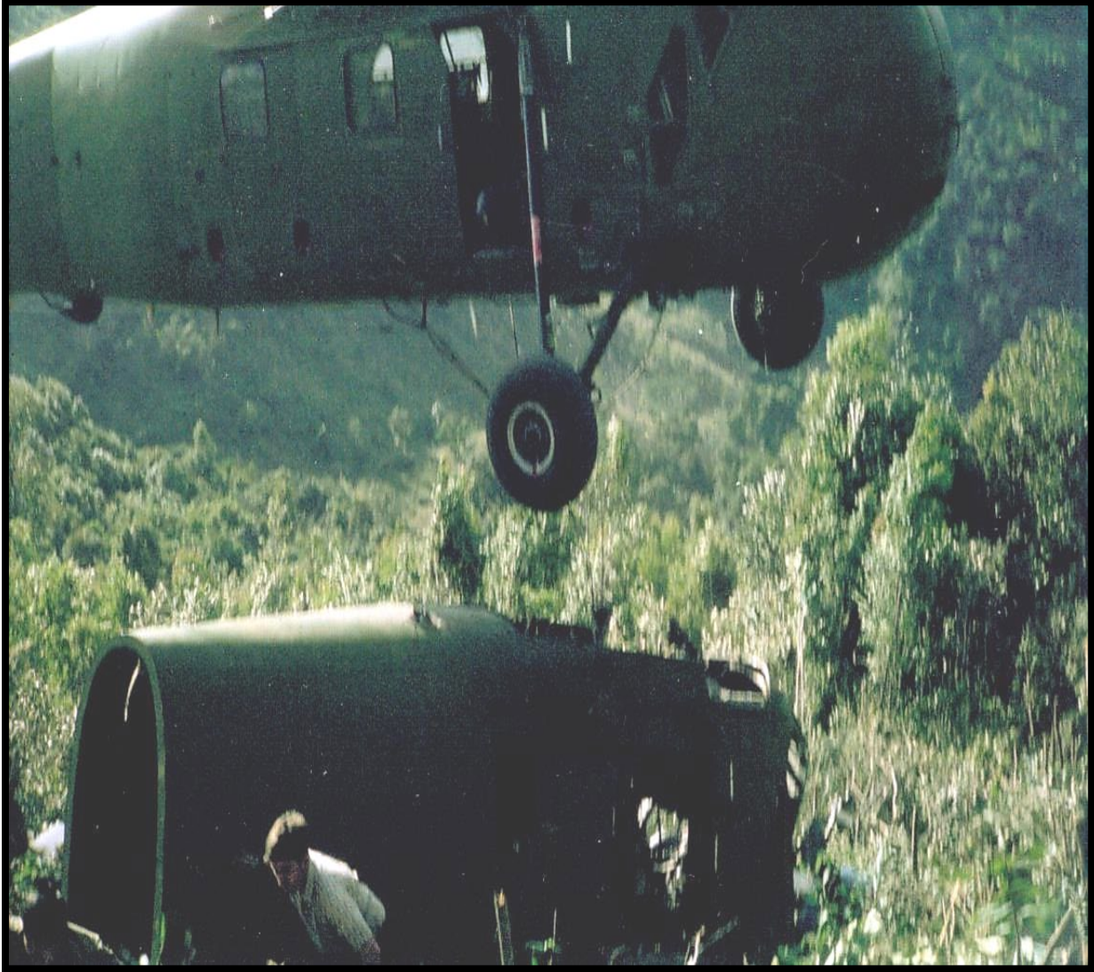
John Fonburg in the process of lifting the Hotel-30 fuselage south to Luang Prabang, where a fixed wing plane could deliver it to Udorn for spare parts or rebuild.
