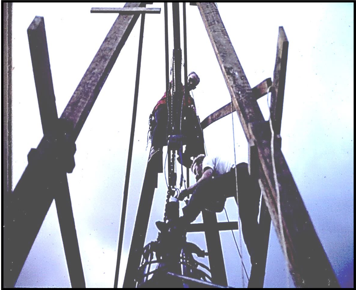
Using discarded wood at Sam Tong for an "A" frame, Pat McCarthy and another mechanic perform a main transmission change on Tom Hoppe's UH-34D.
