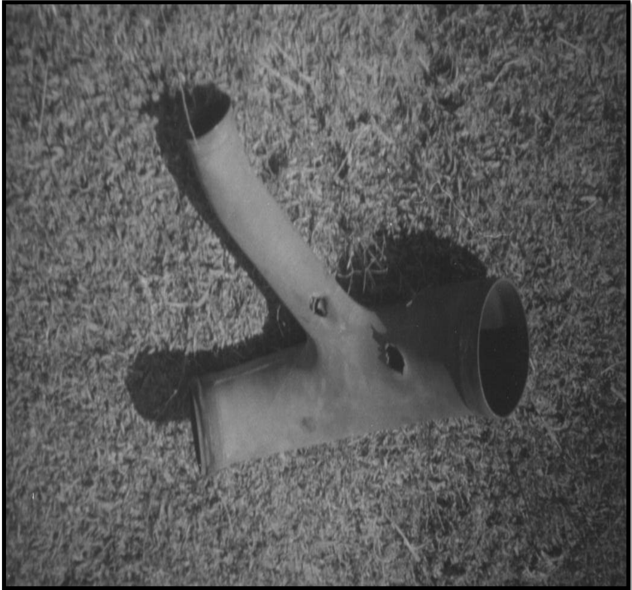
Additional battle damage to Hotel-41 showing holes in the engine exhaust chamber.
