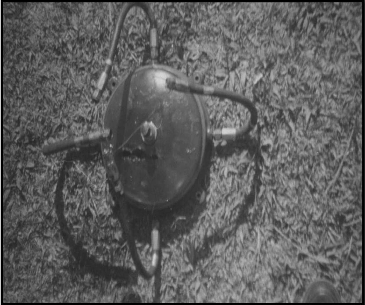
Bullet grazed hydraulic damper reservoir mounted on top of Hotel-41's rotor head.
