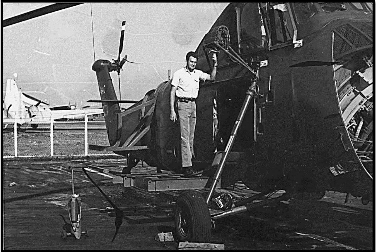
Chief Flight Mechanic Gaza Eiler standing on a locally manufactured apparatus designed to recover crashed aircraft from the field.
