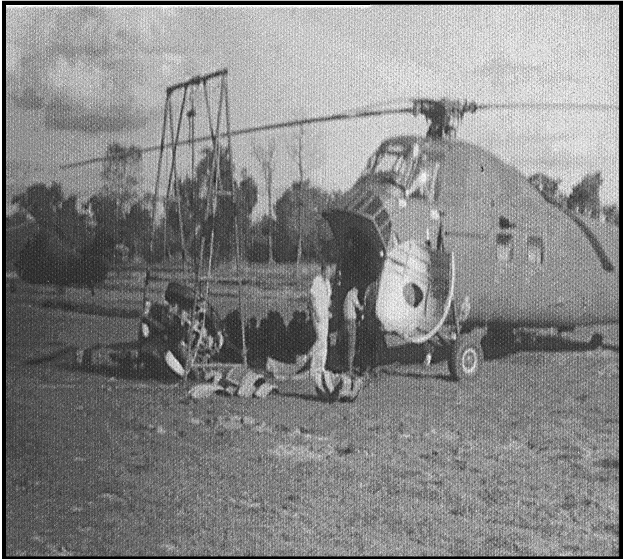
Hotel-37 undergoing a field engine change northeast of Thakhet, Laos. A portable "A" frame and hoist were utilized to effect the change. Stan Wilson supervising a mechanic preparing the tub for the new engine.
