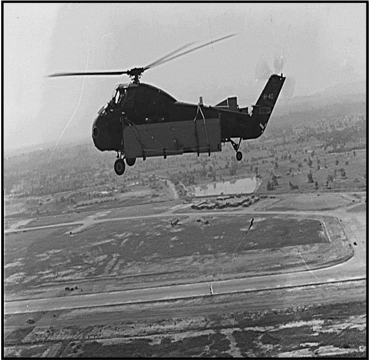
The mounting apparatus on a H-34 for recovered aircraft wings. Burke Collection.
