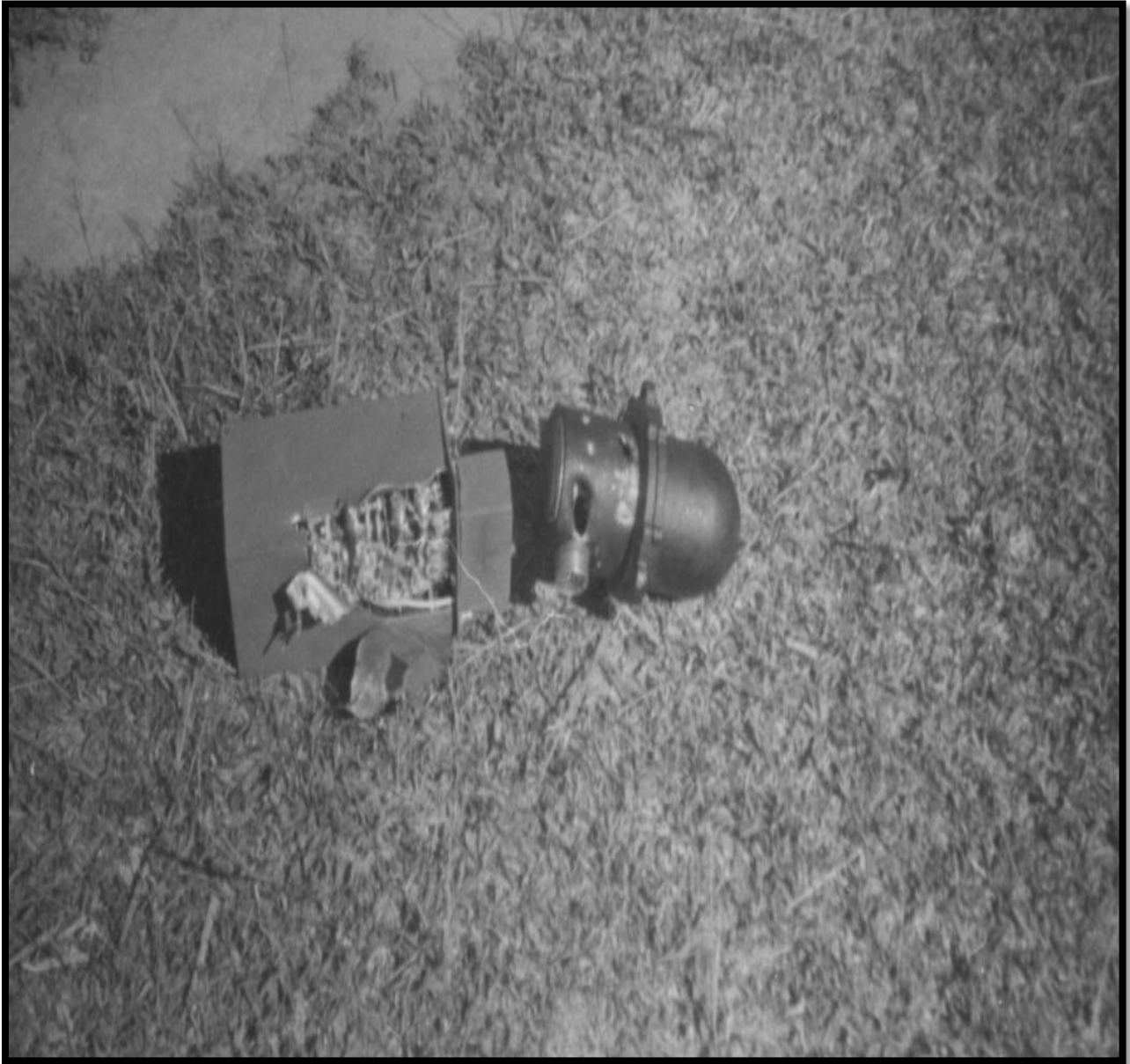
Hotel-41 battle damage to electronics compartment radio and compass components.
