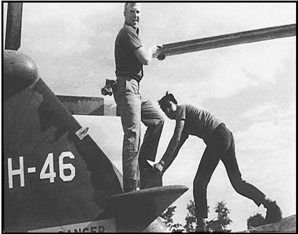
Standing on the tail pylon stabilizer and tail cone, Flight Mechanic Pat McCarthy and an unidentified mechanic inspect Hotel-46's main rotor blades for damage incurred 27 May 1967.
