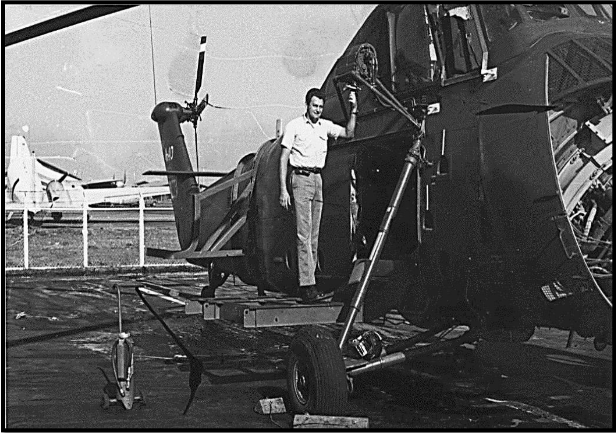
Chief Flight Mechanic Gaza Eiler standing on a portion of the Sikorsky UH-34D small fixed wing recovery apparatus constructed at the Air America Udorn maintenance facility in 1966.
