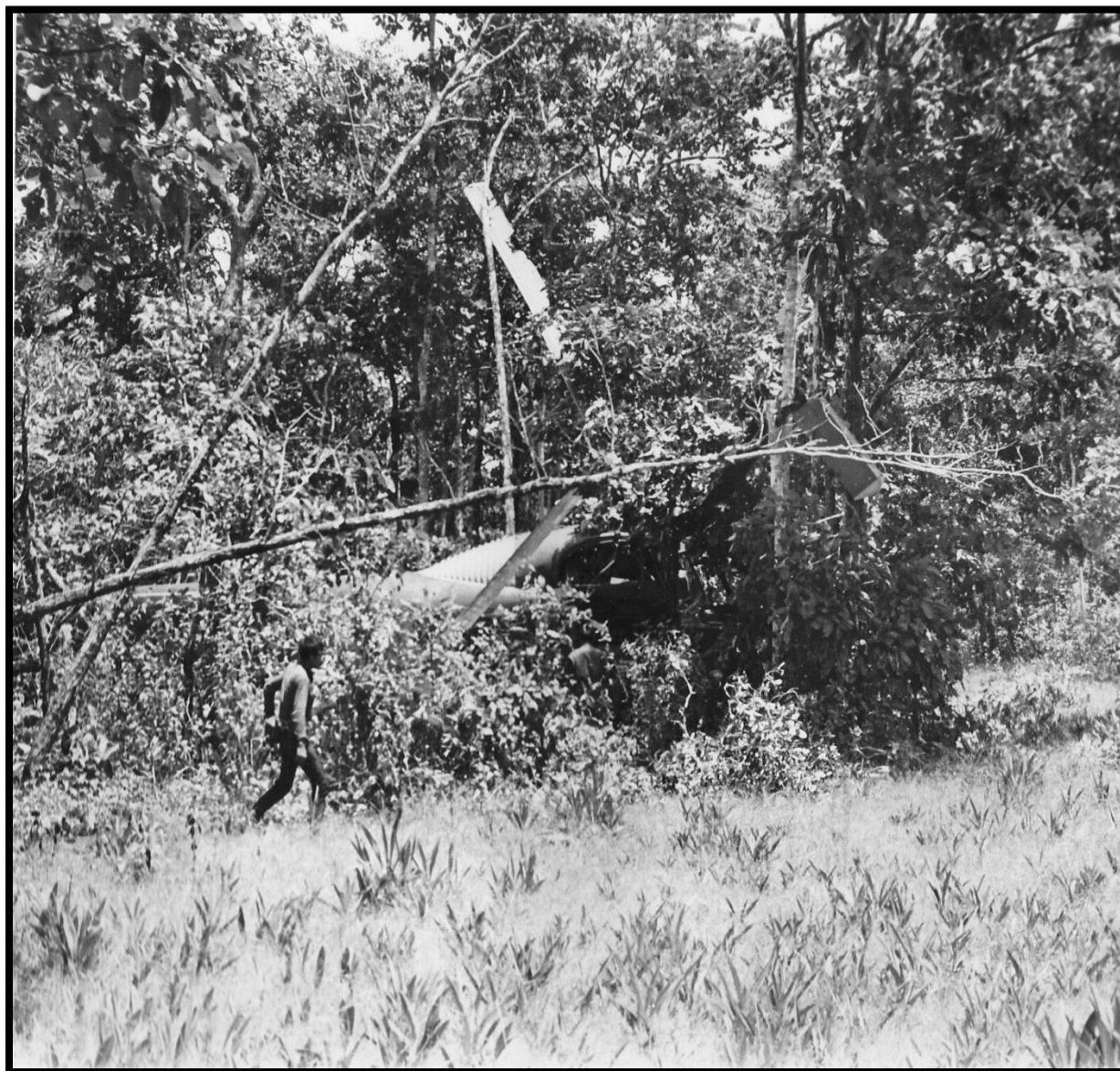
Hotel-39 resting in the trees after a crash landing caused by the complete hydraulic failure.
