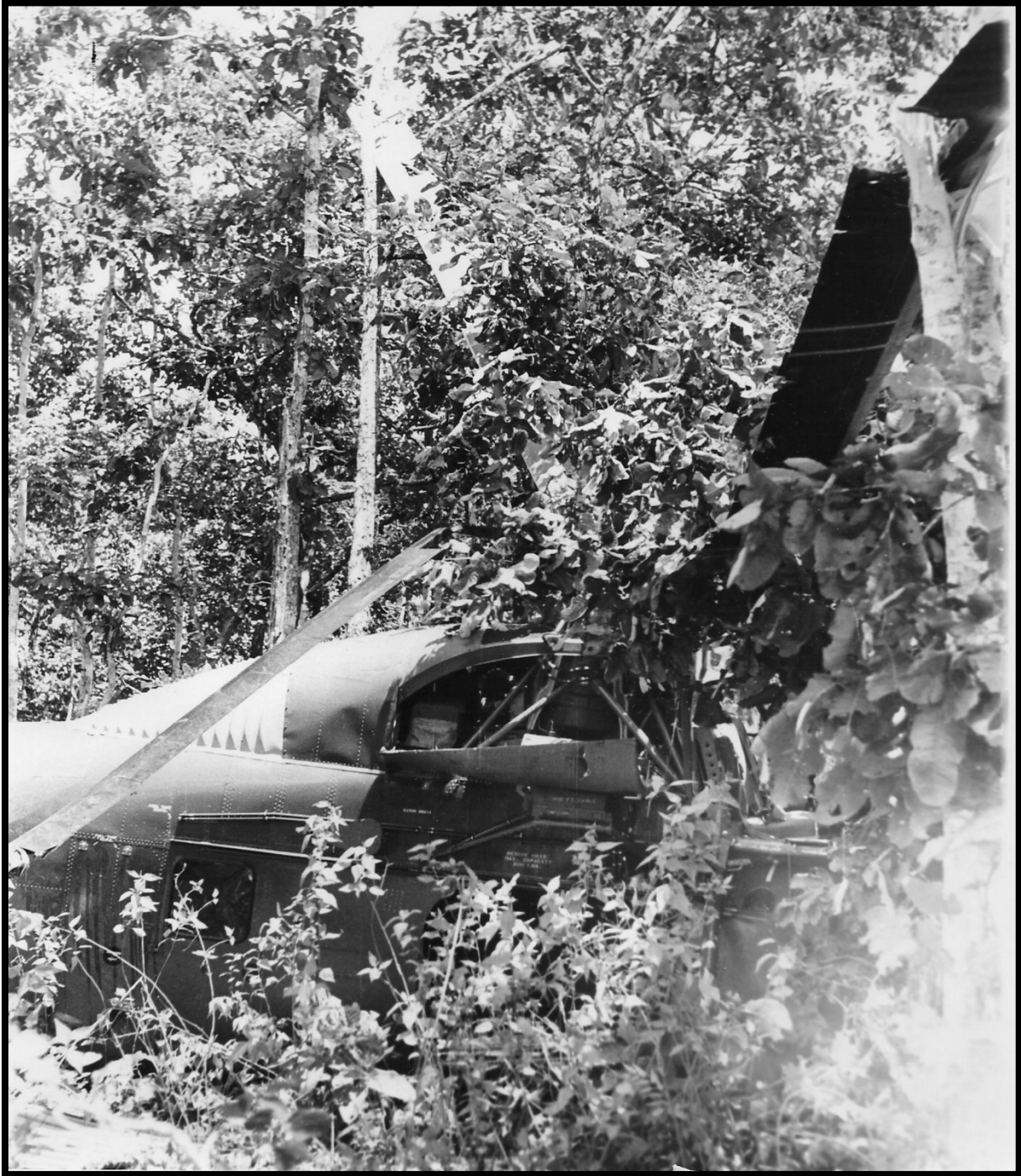
Hotel-39 with the right transmission inspection deck down revealing to the Flight Mechanic a battle damaged "failsafe" three-way hydraulic valve. Splayed and ruined rotor blades display the extent of damage.
