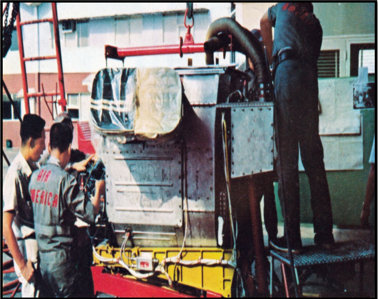
Air America mechanics working on the Pratt and Whitney turbine engines (PT-6) and combining gearbox prior to installation. Left side of a stainless-steel firewall-housed engine is displayed.
