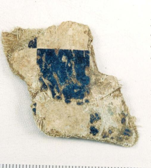
The identified Life Sciences Equipment artifacts all consistently support the conclusion that the involved pilot did not eject prior to crash impact The displayed damage signs, and environmental exposure forms, all support a nonsurvivable (fatal) crash, with no attempt to eject being made > All recovered artifacts are reflective of use in a US Navy A-4 aircraft and escape system, and are consistent with use by a Navy A-4 pilot, during the 1967 time frame
