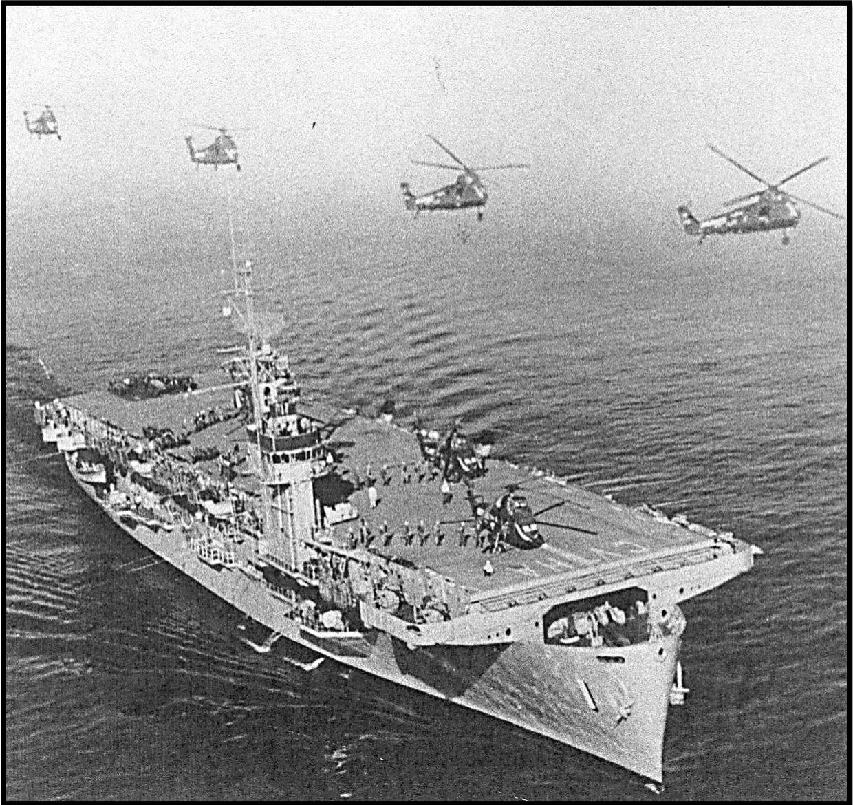
After receiving a "Charlie" signal from pri-fly, a division of HUS-1 pilots in trail formation prepare to turn downwind and land on the LPH, while troops load for a lift. Time was of the essence when recovering on carriers. Therefore, 180-degree breaks were generally performed at two second intervals.
