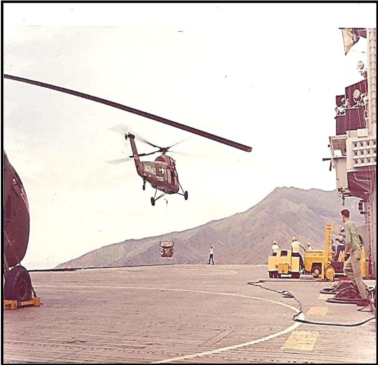
A Yankee Sierra HUS-1 helicopter departing the USS *Thetis Bay* with an external sling load during a ship to shore operation.
